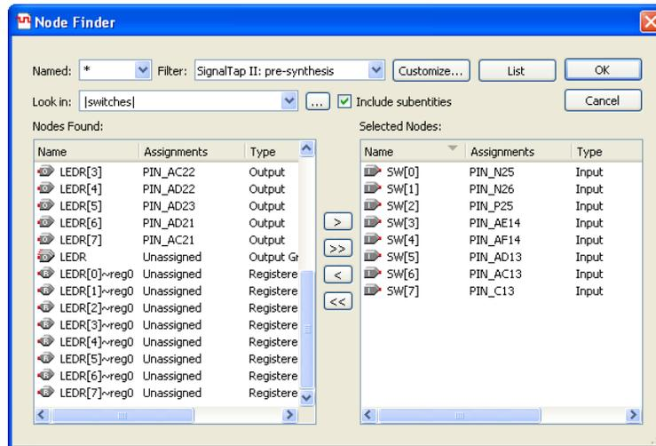
Figure 7. Adding nodes in the Node Finder window on a DE-series board.
