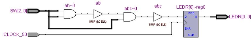
Figure 19. The circuit implemented by the code in Figure 24
