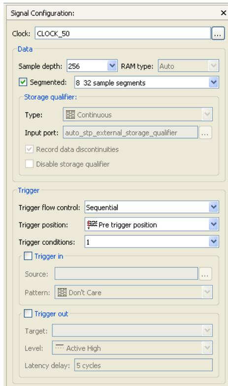
Figure 16. Select Segmented buffer acquisition mode with 8 32 sample segments.
