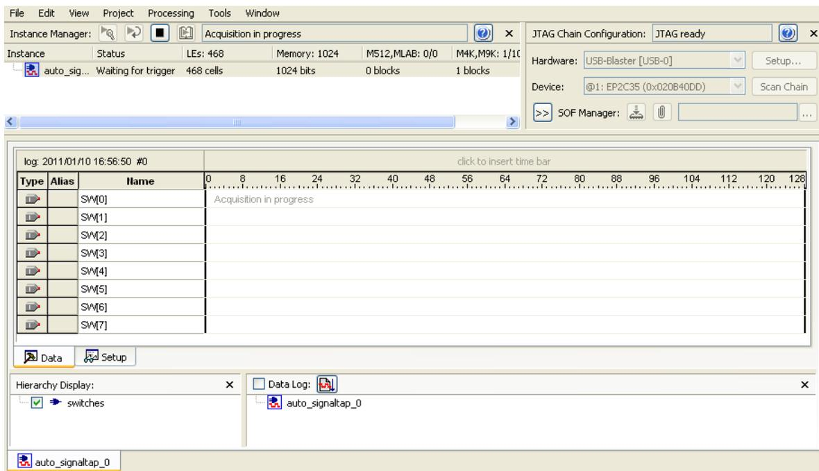
Figure 11. SignalTap II window on a DE-series board after Run Analysis has been clicked.
