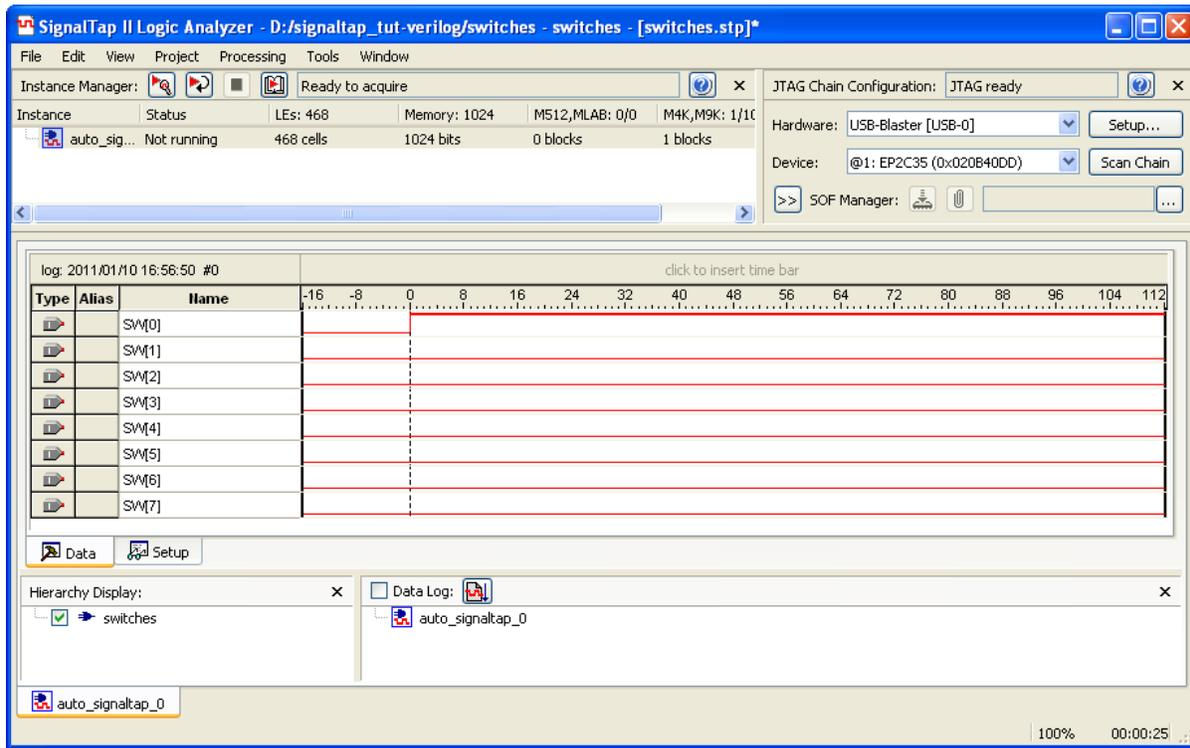
Figure 12. Graphical display of values after trigger condition is met.
