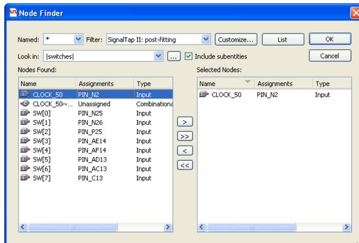
Figure 8. Setting CLOCK\_50 as the clock for the SignalTap instance on a DE-series board.
