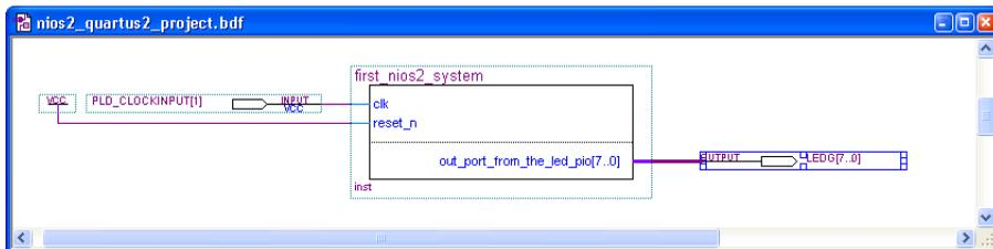
8. If you are targeting a custom board that does not have LEDs, you must delete the **LEDG[7..0]** pins. To delete the pins, perform the following steps:
