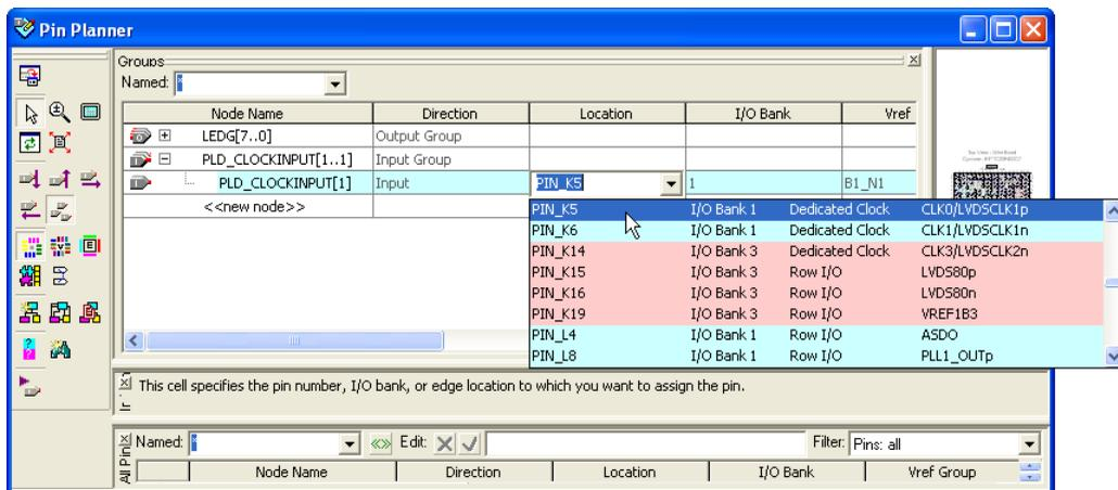
5. If you connected the LED pins in the Board Design File schematic, repeat steps 2 to 4 with **LEDG[7..0]** to assign appropriate pin locations for each of the LED outputs pins: **LEDG[0]**, **LEDG[1]**, **LEDG[2]**, **LEDG[3]**, **LEDG[4]**, **LEDG[5]**, **LEDG[6]**, **LEDG[7]**.
