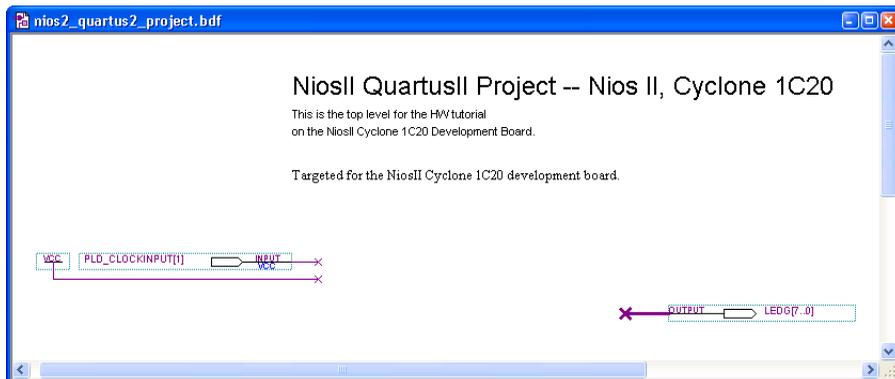
The Block Diagram File contains an input pin for the clock input and eight output pins to drive LEDs on the board. Next, you create a new SOPC Builder system, which you ultimately connect to these pins.
