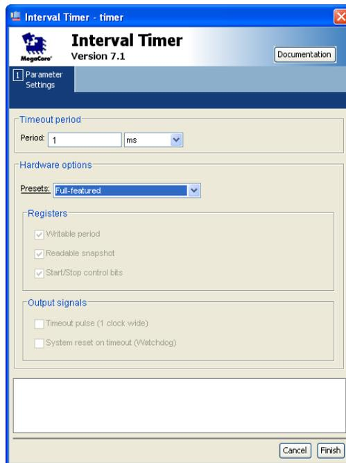
5. Click **Finish**. You return to the SOPC Builder **System Contents** tab, and an instance of the interval timer named **timer** now appears in the table of available components.
