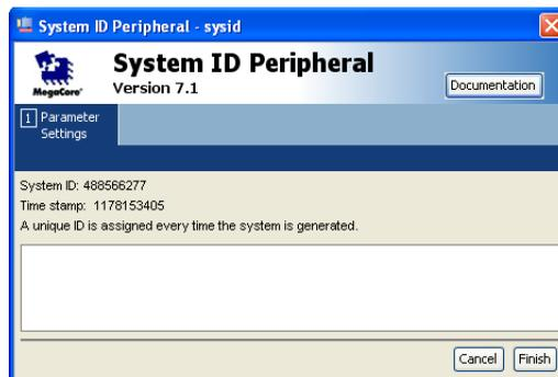
3. Click **Finish**. You return to the SOPC Builder **System Contents** tab, and an instance of the system ID peripheral named **sysid** now appears in the table of available components.
