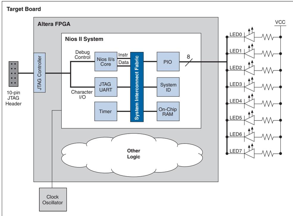
As shown in Figure 1-1, other logic can exist within the FPGA alongside the Nios II system. In fact, most FPGA designs with a Nios II system also include other logic. A Nios II system can interact with other on-chip logic, depending on the needs of the overall system. For the sake of simplicity, the example design in this tutorial does not include other logic in the FPGA.
