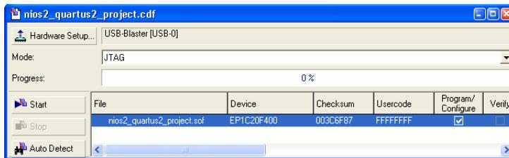
At this point, the Nios II system is configured and alive in the FPGA, but it does not yet have a program in memory to execute.
