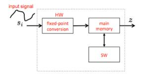
point converter, which samples the input signal and stores the resultant samples in fixed-point representation in the main memory as illustrated in the figure. The fixed-point representation is 8-bit total with 2 bits for the fractional part. The SW component, which executes on a 32-bit soft processor, is a simple SW routine that reads the samples from the memory and computes z.
