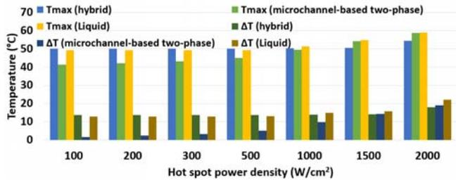
Fig. 8: Comparison of cooling performance among hybrid cooling, microchannel-based two-phase cooling, and liquid cooling via microchannels.
