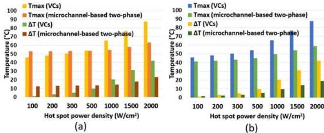
Fig. 9: Comparison of cooling performance between two-phase VCs with micropillar evaporators and microchannel-based two-phase cooling of various input mass fluxes: (a) 100 kg/m<sup>2</sup>s, (b) 560 kg/m<sup>2</sup>s.
