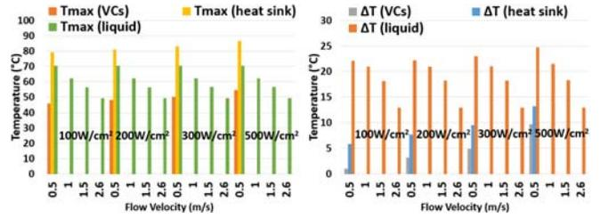
Fig. 6: Comparison of cooling performance among the conventional heat sink, two-phase VCs with micropillar evaporators, and liquid cooling via microchannels.
