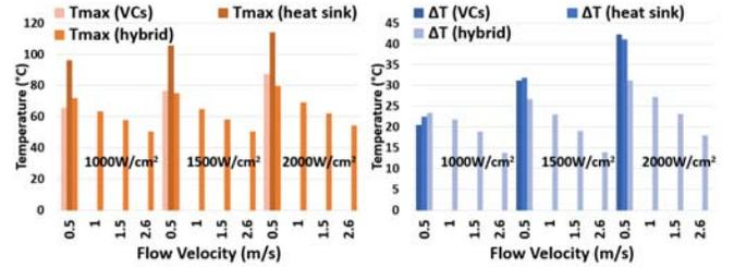
Fig. 7: Comparison of cooling performance among the conventional heat sink, two-phase VCs with micropillar evaporators, and hybrid cooling when TEC current = 7 A.
