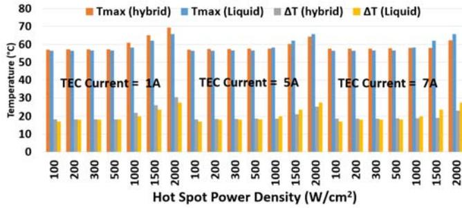
Fig. 5: Comparison of cooling performance between hybrid cooling and liquid cooling via microchannels, when liquid flow velocity = 1.5 m/s.
