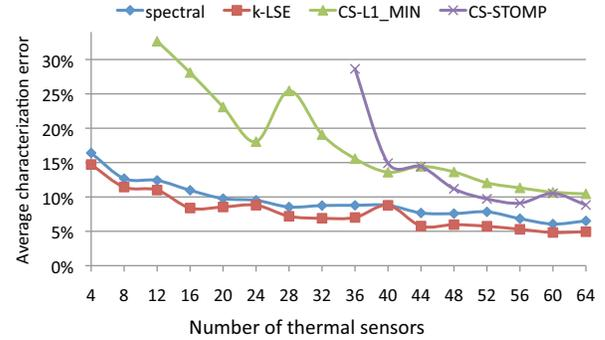
**Figure 7: Average error in full thermal characterization using various temperature reconstruction methods.**
