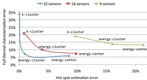
**Figure 10: Hot spot error and full thermal characterization error as a function of thermal sensor placement methodology. k-LSE method is used for full thermal reconstruction.**
