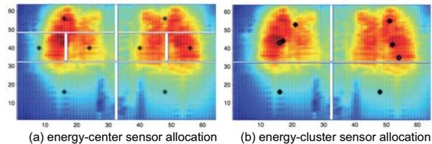
**Figure 3: Proposed thermal sensor allocation based on spectral energy density.**
