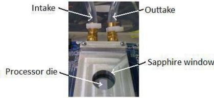
**Figure 6: Setup for oil-based infrared transparent heat spreader.**
