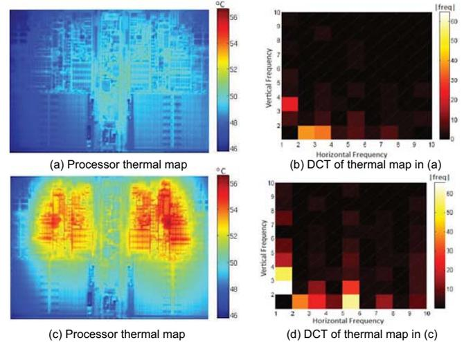
**Figure 1: Thermal maps of Athlon dual II processor and their corresponding DCT frequency-domain representations.**
