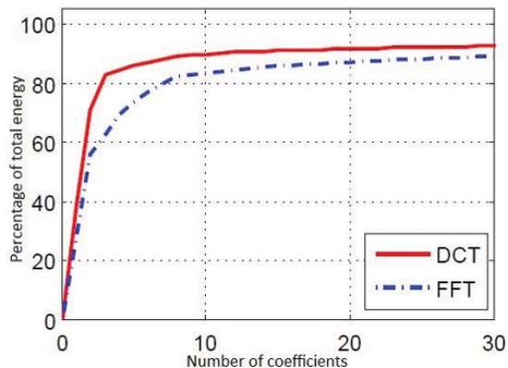
**Figure 2: Fraction of signal energy captured as a function of the number of frequency-domain coefficients.**
