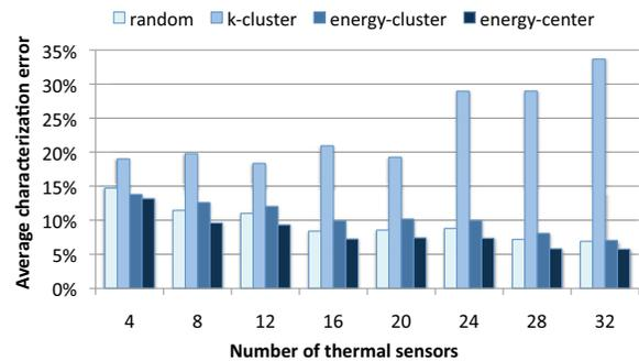
**Figure 8: Average error in full thermal characterization using the *k-LSE* for various sensor allocation strategies.**
