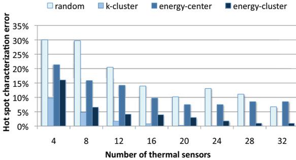
**Figure 9: Average error in hot spot estimation using various number of sensors and sensor allocation strategies.**
